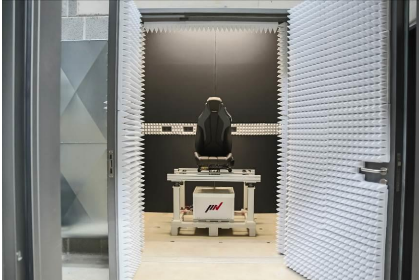
Caption: An acoustic shaker is available for the analysis of noise interference, allowing critical effects such as rattling or creaking to be more closely investigated.
