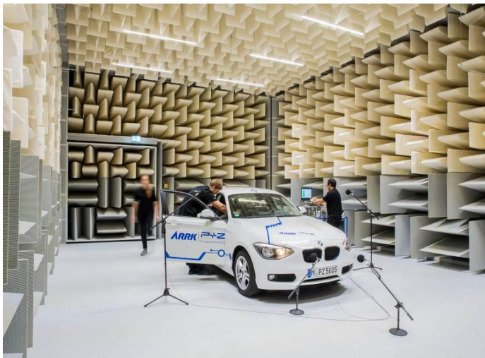
Caption: The new semi-open room is optimally designed for testing, allowing the noise emitted by entire vehicles as well as individual components and modules to be tested down to a lower frequency limit of 50 Hz. Other machines, technical devices, household goods and consumer electronics can also be tested.
